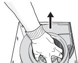
Remove wiring panel from fan housing (if already installed).
