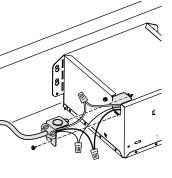
details. Use black screw (from parts bag) to secure wiring plate to fan housing. Re-install wiring panel and secure with screw from parts bag.
