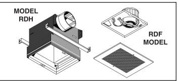
Dependable, high performance ventilation fan with attached radiation damper and attractive metal grille.
