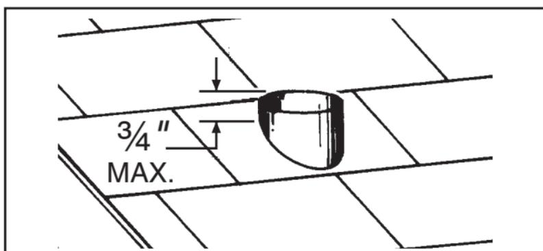
1. Cut hole in roof approximately  $\frac{1}{2}$ " larger than ductwork.
