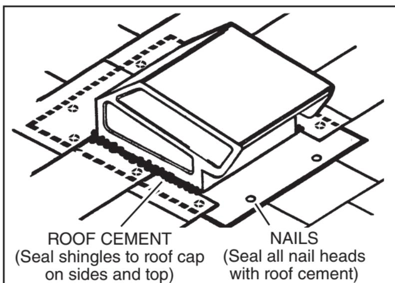
6. Carefully lift shingles and slide back flange of roof cap under shingles. Nail flange to roof under shingles at top and two sides. Nail directly to roof at bottom.
