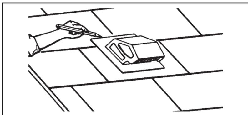
4. Lay roof cap over ductwork and trace outline of roof flange onto shingles.
