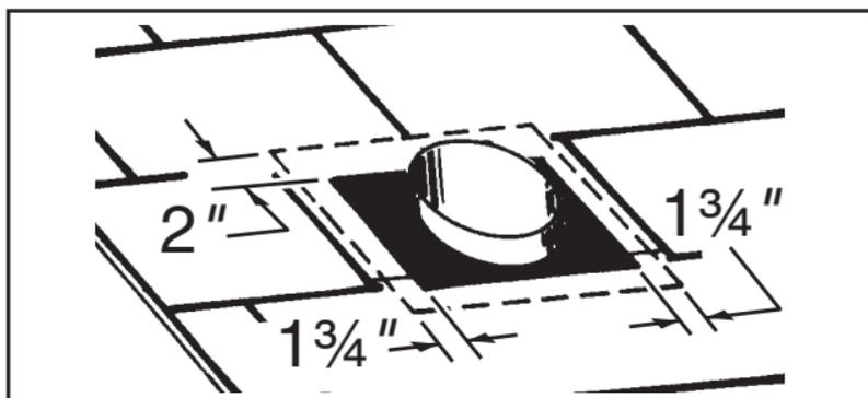
5. Trim shingles as shown, so they will fit snugly around hood of roof cap when installed. Seal all around duct with roof cement.
