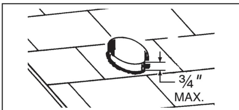
3. Trim ductwork parallel to roof pitch.
