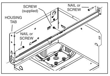
3. NAIL or SCREW the brackets to the ceiling framing (joists, trusses, etc.).
