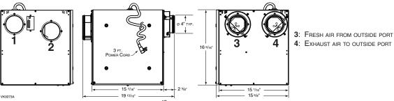
NOTE: ALL UNITS PORTS WERE CREATED TO BE CONNECTED TO DUCTS HAVING A MINIMUM OF 4" DIAMETER, BUT IF NEED BE, THEY CAN BE CONNECTED TO BIGGER SIZED DUCTS BY USING AN APPROPRIATE TRANSITION (E.G.: 4" DIAMETER TO 5" DIAMETER TRANSITION).
