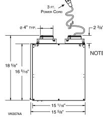
NOTE: ALL UNITS PORTS WERE CREATED TO BE CONNECTED TO DUCTS HAVING A MINIMUM OF 4" DIAMETER, BUT IF NEED BE, THEY CAN BE CONNECTED TO BIGGER SIZED DUCTS BY USING AN APPROPRIATE TRANSITION (E.G.: 4" DIAMETER TO 5" DIAMETER TRANSITION).
