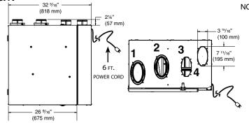
NOTE: ALL UNITS PORTS WERE CREATED TO BE CONNECTED TO DUCTS HAVING A MINIMUM OF 6" DIAMETER, BUT IF NEED BE. THEY CAN BE CONNECTED TO BIGGER SIZED DUCTS BY USING AN APPROPRIATE TRANSITION (E.G.: 6" DIAMETER TO 7" DIAMETER TRANSITION).
